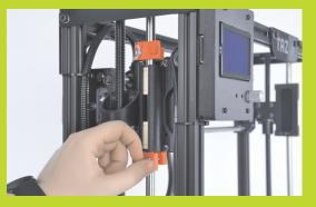
Remove the red protective packing clips from the Z and Y axis smooth rods.
