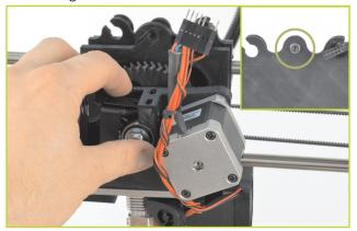
Plug in the tool head. Note the pin orientation: The tool head connector should have a small gap in the pins on the right-hand side. When the tool head is fully seated, the connectors should fit flush against each other.
