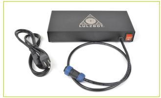
Locate the blue 24VDC output cable plug from the power supply. Connect the blue power supply plug into the keyed power supply connector on the printer electronics enclosure. Once the plug is pushed in completely, turn the locking
