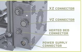
**CONT.** The top-most connector matches the large straight plug from the XZ cable. The next connector down matches the large angled plug from the YZ cable. The third connector matches the smallest plug, from the heated bed cable.
