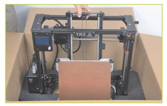
Carefully remove the entire printer frame from the box and set it on a sturdy, flat surface near an electrical outlet. Now you are ready to set up your LulzBot<sup>™</sup> TAZ 3D printer!
