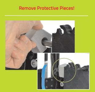
Locate and remove the gray foam block used to hold the X axis carriage in place during shipping.
