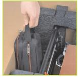
Keeping the printer in the box, grab the printer by its black side frames. Pick up and rotate the printer 90 degrees, setting it upright within the box. Verify that the part of the frame with the LCD and TAZ name plate are up. Remove the top black foam.
