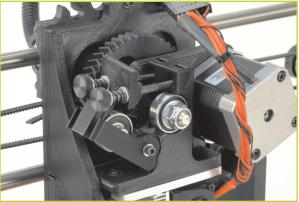
C Once the filament extrudes a small amount out of the nozzle, raise the idler and slide the two idler bolts and plate back into place. Tighten the two idler bolts. Tighten the two screws until the top of the thumbscrews are about 10mm (0.4 inches) away from the plastic clip.
