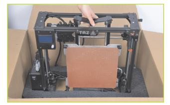
**B** Rotate the print bed assembly (Y axis), tilting the bottom toward front of box. Lower the print bed assembly (Y axis) into the box so it is parallel with printer frame, then it lift out and set it aside.
