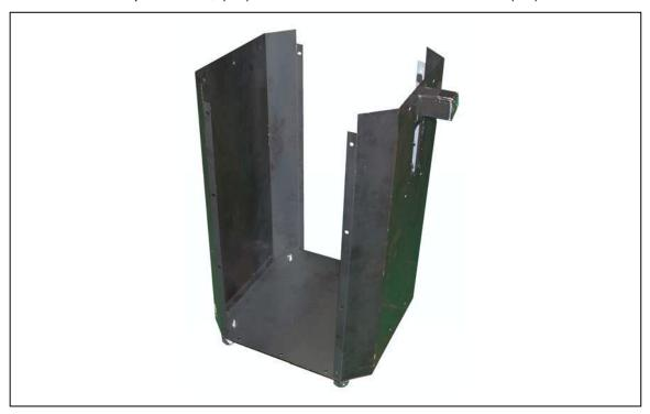
Step Nineteen: Assemble the side panels to the drum using (6) 5/16"\*5/8" Philip hd bolts, (12) 5/16"\*OD18\*2t flat washers and (6) 5/16" nuts to secure the base. And then use (16) 5/16"\*5/8" Philip hd bolts, (16) 5/16"\*OD18\*2t flat washers and (16) 5/16" nuts to secure the panels to each other.
