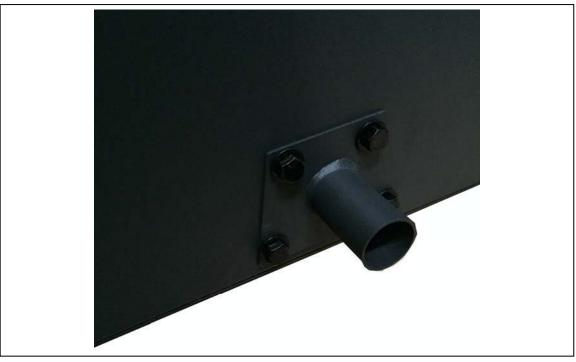
Step Twenty Three: Attach the  $\emptyset$ 1-1/4"x0.8M black flex hose to the drum vacuum suction tube and use the  $\emptyset$ 1-1/4" hose clamp to tighten and secure the black flex hose in place.
