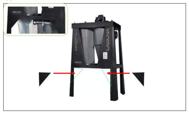
Step Five: Secure the (2) triangular cover plates to the back of the unit. Use (8) 5/16"\*1" hex bolts, (16) 5/16"\*OD18\*2t flat washers and (8) lock nuts.
