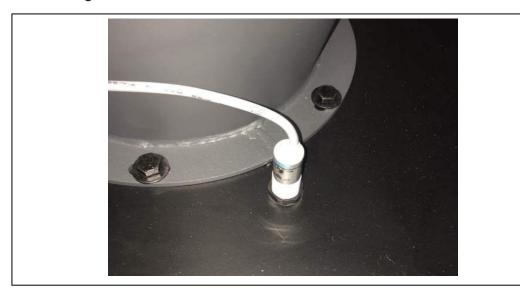
Step Thirteen: Make sure that the proximity sensor is not thread in too deeply into the drum lid. As this will create interference when the drum is inserted and may hit the proximity sensor creating damage.
