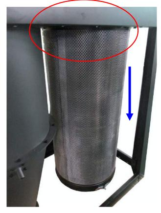
4. With the canister filter removed use a compressed air gun to thoroughly clean between the pleats, both inside and outside.
