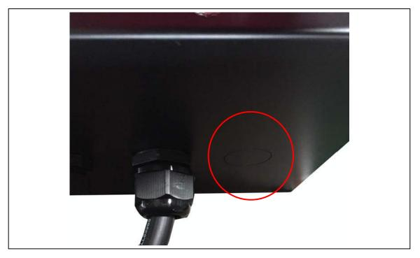
Step Thirty One: Thread the power cord through the hole in the control box and connect to L1 and L2 terminal.
