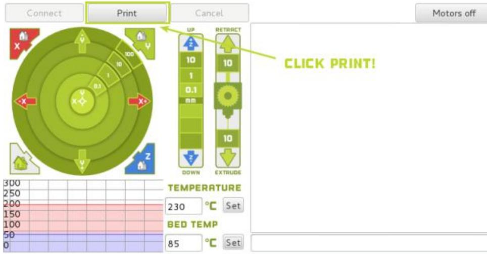
**10B** Your LulzBot TAZ will first cool down and move to the front of the bed to clean off its nozzle. After cleaning, your LulzBot TAZ will then conduct an automated bed-leveling sequence, heat up to final temperature, and start printing. This process can take up to five minutes.
