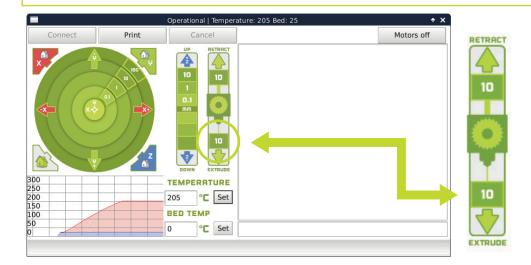
**10B** If you do not see filament coming through the nozzle and the drive gear stops moving, click the **Extrude 10** button once more and wait. Repeat as needed until you see consistent and repeatable extrusion.
