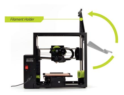
**8B** We strongly recommend using the included PLA filament sample for your first rocktopus print. Mount the PLA filament sample on the filament holder so the filament can feed down into the tool head.
