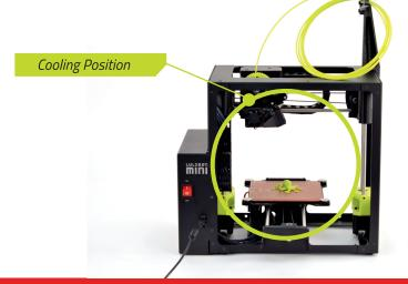
Your printer is now actively cooling. Do not attempt to remove your 3D printed object before the print bed moves forward. Attempting to do so could either burn your skin on the hot end or print bed, damage your printer, or damage your 3D printed object.
