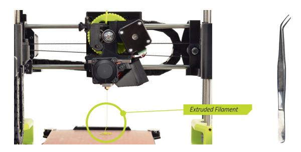
**10C** Wait ten seconds for the filament to cool, then remove the extruded filament with the included tweezers.
