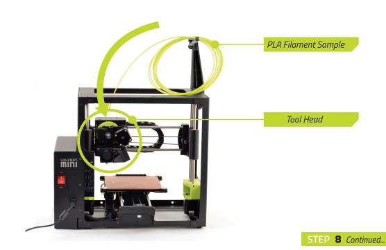
**8**C Locate the feed hole in the extruder body where you removed the loaded filament during Step 7. Filament feeds through this hole and down into the hot end for printing.
