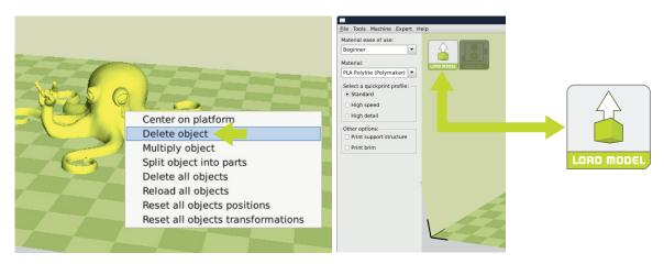
**14F** With your new object set, double check that your material and print profile selections match the filament you are using, and the quality that you want. When your file is ready for printing, press **Control**, and then in the Printer Interface window click **Print**.
