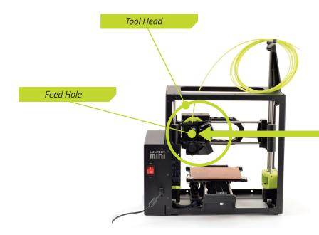
**8D** Make sure the idler retainer is touching the springs so it is out of the way. Then push the PLA filament down into the feed hole in the extruder body and through the hot end until a small amount of filament comes out of the tip of the nozzle.
