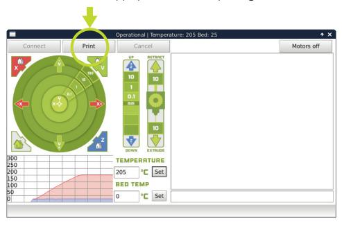
**11B** Your LulzBot Mini will first move its tool head to the top left corner and allow the hot end to cool down prior to starting its cleaning process. Depending on ambient air temperature, this can take two to five minutes.
