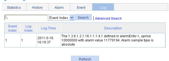
In this example, event 1 has generated one log, which is triggered because the alarm value (11779194) exceeds the rising threshold (10000000). The sampling type is absolute.
