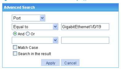
2. Click the **Advanced Search** link, specify the search criteria on the advanced search page as shown in Figure 14, and click **Apply**. The ARP entries with interface being GigabitEthernet1/0/19 and IP address range being 192.168.1.50 to 192.168.1.59 are displayed as shown in Figure 15.
