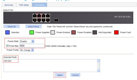
After the configuration takes effect, the IP telephones and the AP are powered and can work correctly.
